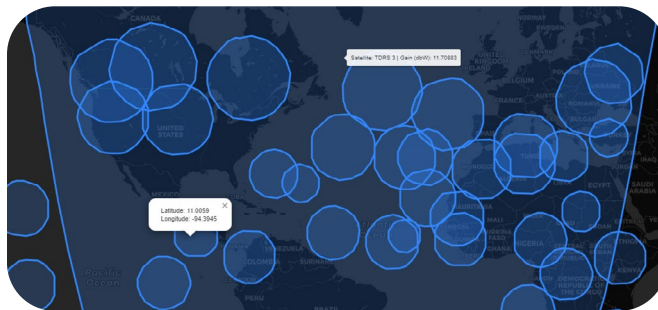
Multi-orbit projection of a single NADIR beam for TDRS 3 and 100 Starlink Satellites (8ms per timestep)
