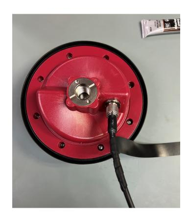
Cover as much of the connector as possible. Stretch the tape into the threads above the connector
