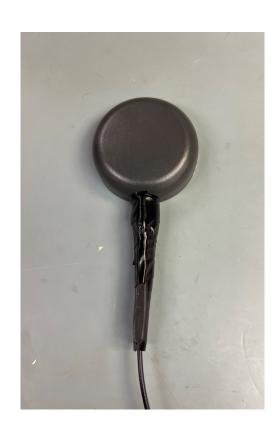
• When applying the mastic tape be sure to seal the interface between the plastic radome and the SMA connector.
