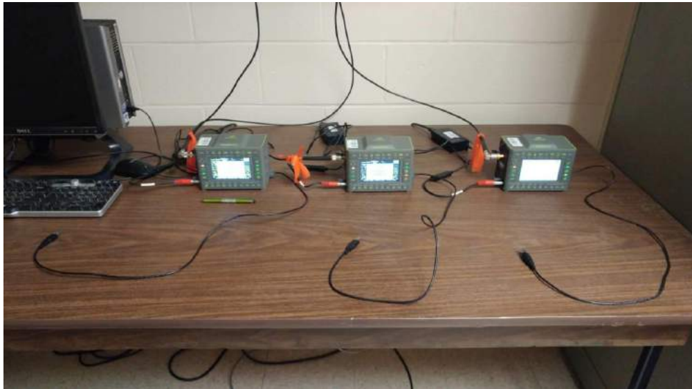
Figure 4: Javad Triumph LS receivers connected to the Tallysman VP6000, AOA choke-ring, and Leica AX1203+ antennas on the roof of Gillin Hall.
