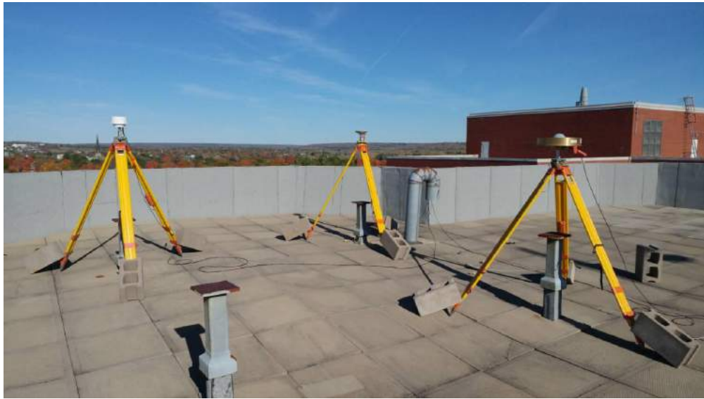
Figure 3: Tallysman VeraPhase VP6000 (left), Leica AX1203+ (middle), and AOA choke-ring (right) antennas set on tripods at a 1.5-metre height on DOY 287-289.
