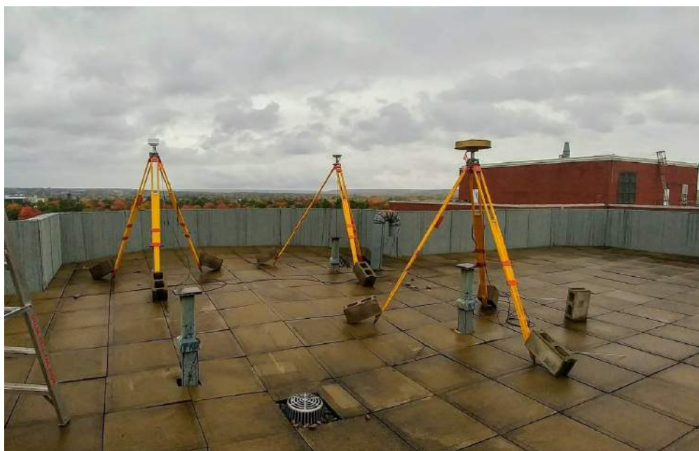
Figure 2: Tallysman VeraPhase VP6000 (left), Leica AX1203+ (middle), and AOA choke-ring (right) antennas set on tripods at 2-metres height on DOY 283-285.
