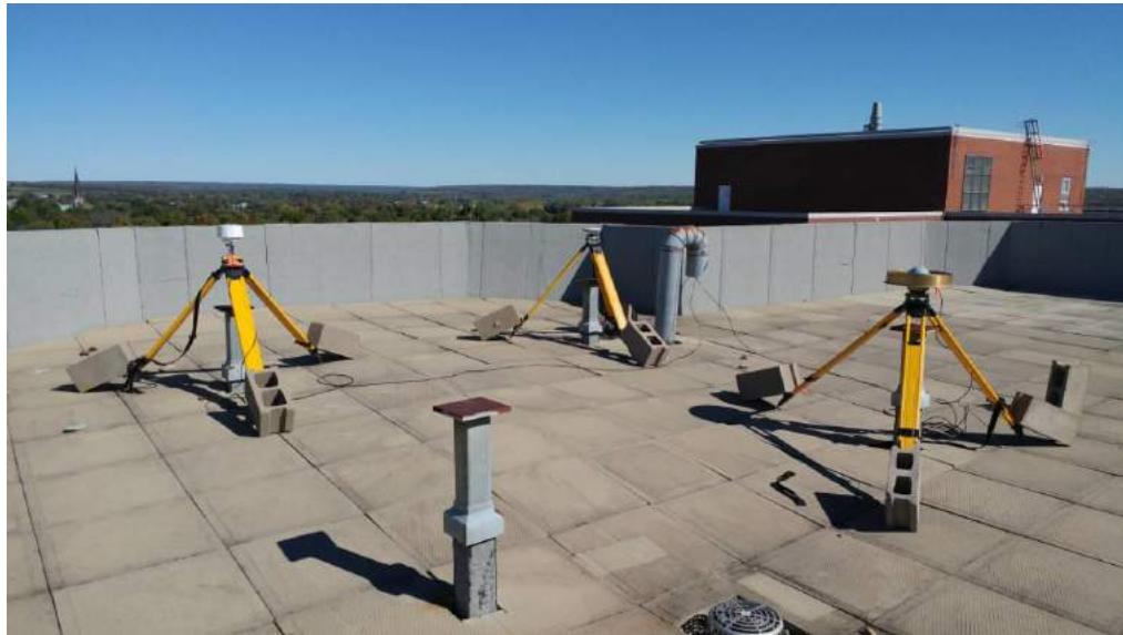
Figure 1: Tallysman VeraPhase VP6000 (left), Leica AX1203+ (middle), and AOA choke-ring (right) antennas set on tripods at a 1-metre height on DOY 278-280.
